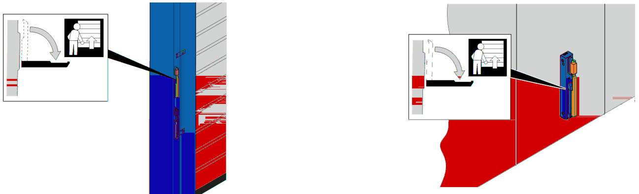
Fig. 15: Manual release lever fitted on the side frame (left) and on a separate console (right)
