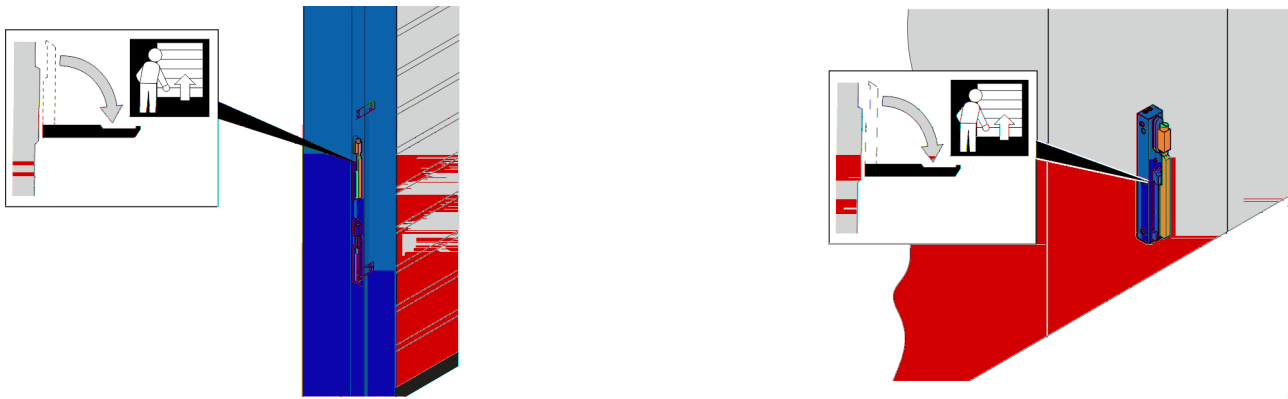
Fig. 12: Manual release lever on the side frame (left) and on a separate console (right)
