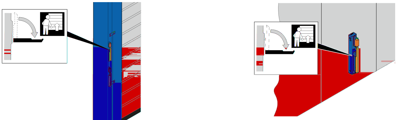
Fig. 21: Manual release lever on the side frame (left) and on a separate console (right)
