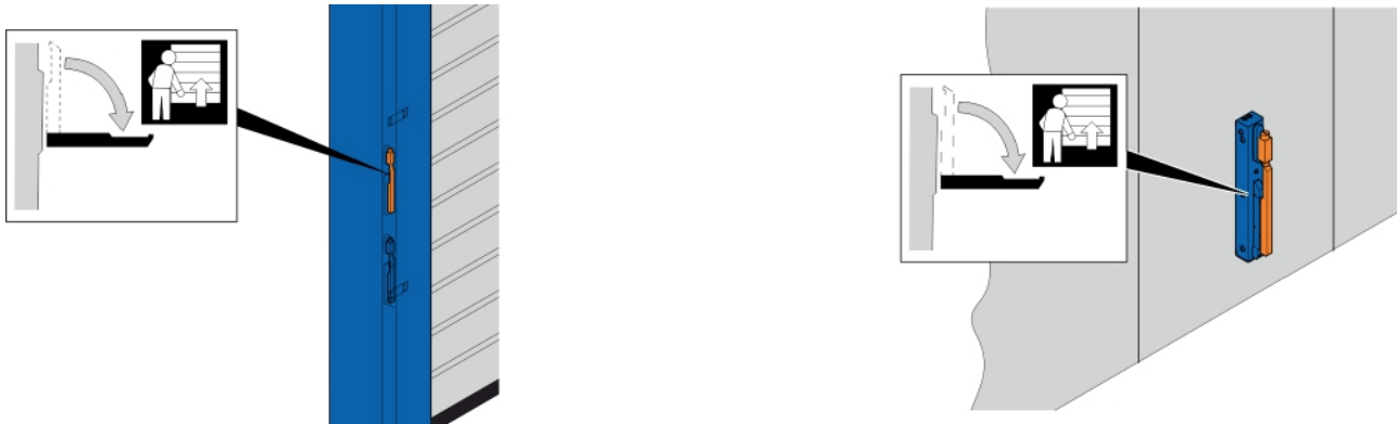
Fig. 14: Manual release lever on the side frame (left) and on a separate console (right)
