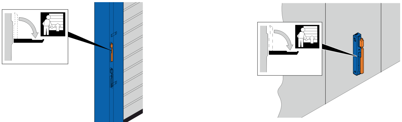
Fig. 24: Manual release lever on the side frame (left) and on a separate console (right)
