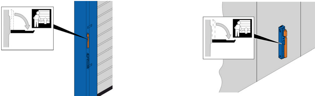
Fig. 17: Manual release lever on the side frame (left) and on a separate console (right)
