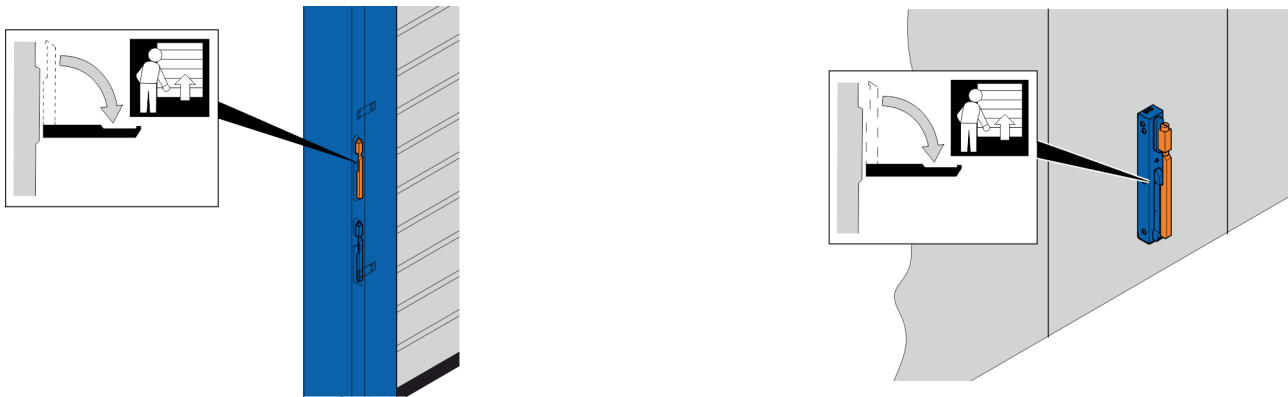
Fig. 12: Manual release lever on the side frame (left) and on a separate console (right)
