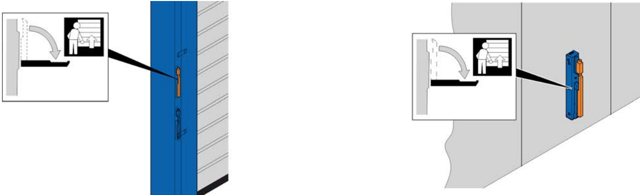
Fig. 23: Emergency lever on the side frame (left side) and on the console (right side)
